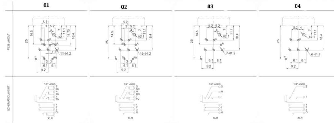
**Electrical Specification:**Contact Resistance:  $\leq 0.03\Omega$ Insulation Resistance:  $\geq 100M\Omega$
