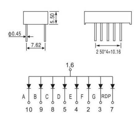
Note: All dimensions in the figure are in mm; The size error margin not indicated is  $\pm 0.25$ mm;
